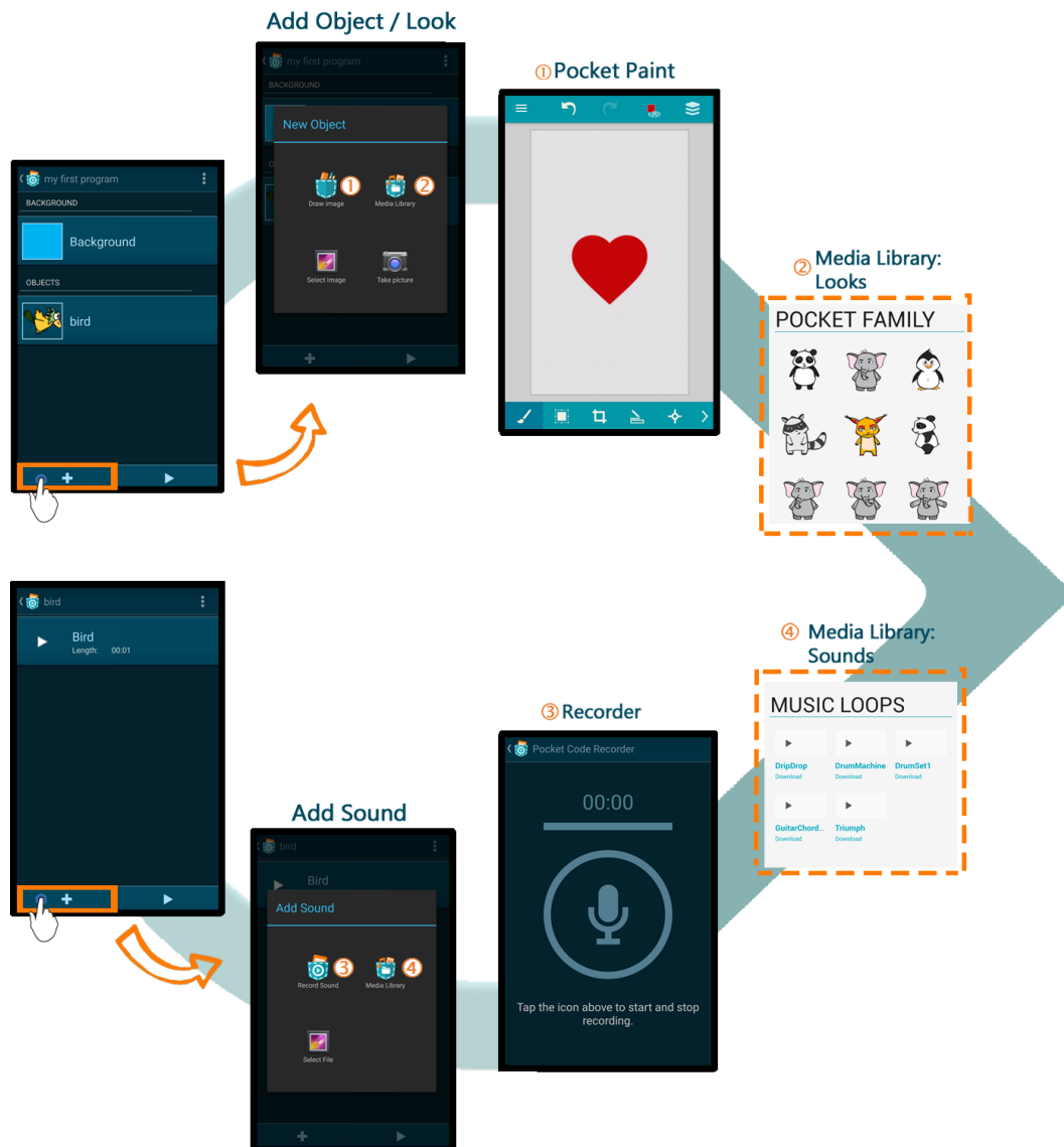
Figure 3.6.: Pocket Code's UI: add a lookobject or add a sound with the "+" sign.
