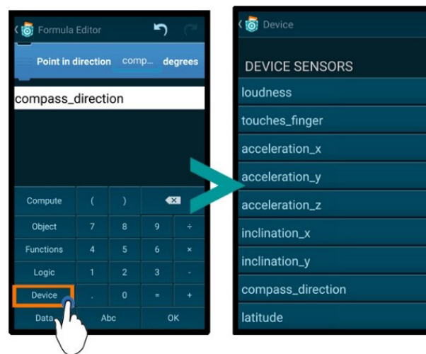
Figure 3.8.: Formula Editor: a. The value for the direction can be defined as a constant or, a sensor can be chosen by tapping "Device"; b. Available sensors which can be used.
